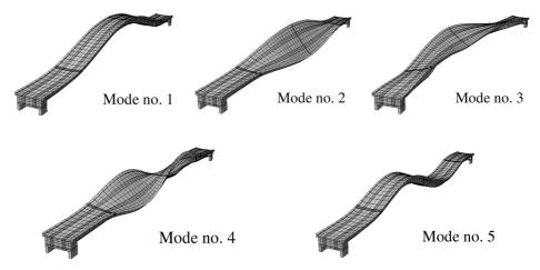
Fig. 5. The mode shapes of the footbridge
