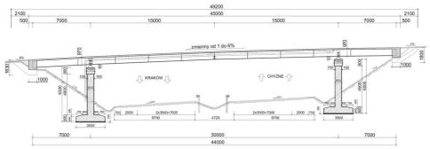
Fig. 1. Longitudinal section of the footbridge in Mogilany
