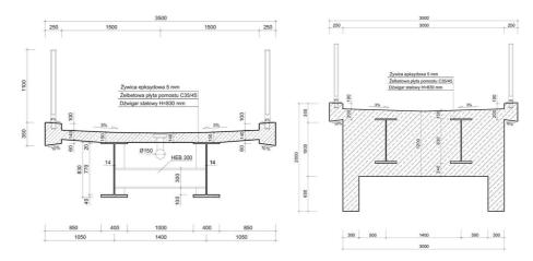
Fig. 2. Cross sections of the footbridge a) mid-span, b) near the abutments
