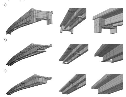
Fig. 4. Variants of computational models: a) F-1 - model with integral abutments, b) F-2 - model with tension rocker bearings, c) F-3 - model with concrete side spans
